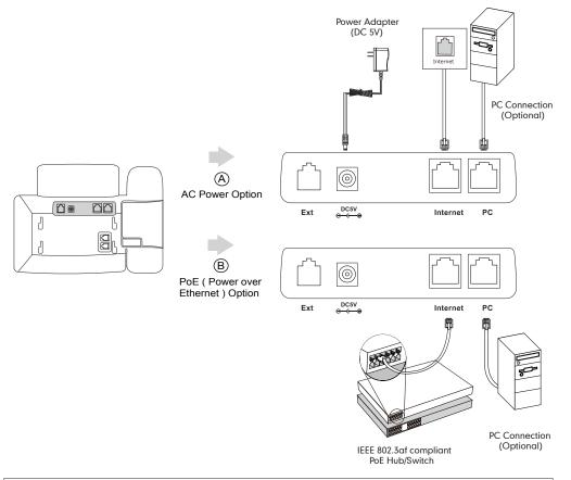
**Note:** If inline power (PoE) is provided, you do not need to connect the power adapter. Make sure the Ethernet cable and hub/switch are PoE compliant.
